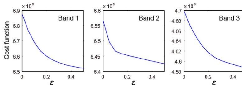
Fig. 4. Effect of relative change in onboard spectral response transform matrix ( $\epsilon$ ) on cost function.
