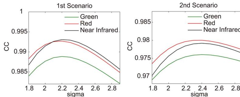
Fig. 3. Correlation coefficient of sharpness between two low spatial-resolution multispectral images generated from Hyperion and ASTER data.
