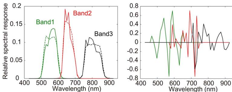
Fig. 5. Result of estimating relative spectral response function between ASTER and Hyperion. Pre-launch (dashed line on left), convex optimization (solid line on left) and least-squares (right).
