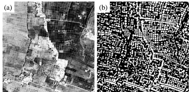
Fig. 3. (a) Reflectance data (band 110), (b) segmentation of paddy field
