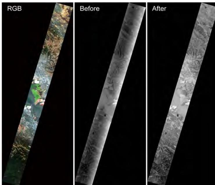
Figure 8. Radiance difference between bands 40 and 42 before (middle) and after (right) smile correction in L1G data.
