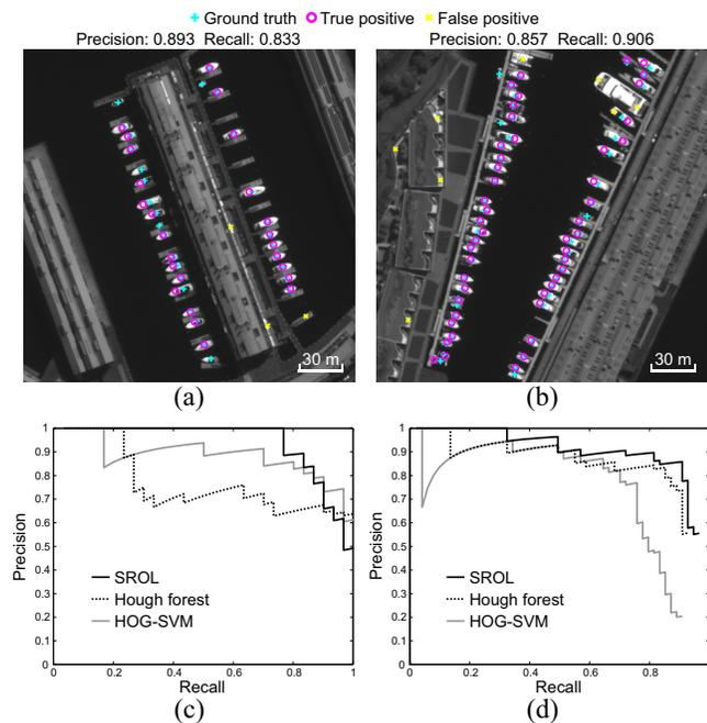
**Fig. 4.** Ship detection results and precision-recall curves for two test images.
