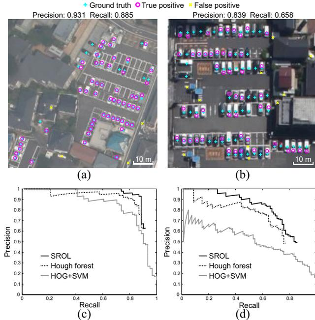
**Fig. 3.** Car detection results and precision-recall curves for two test images.
